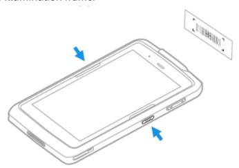
4. Release the Scan button when the computer beeps, and the Scan Status LED briefly turns on. The bar code information is entered into the application in use.
